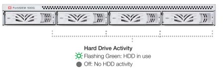
Note: Only 1 hard disk is installed and supported.
